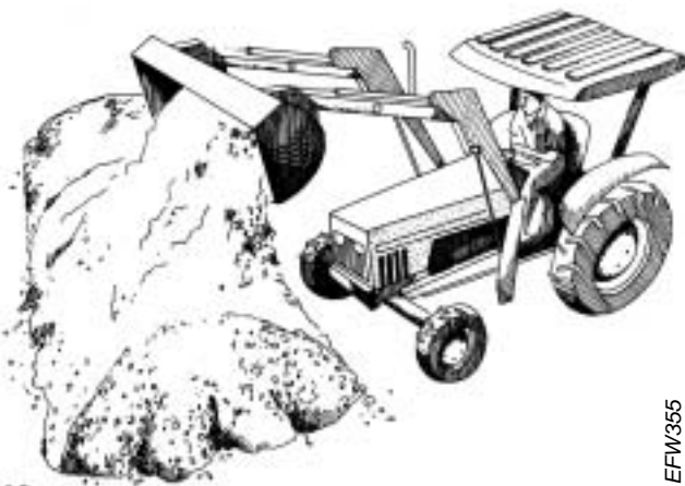
Figure 17. A front-end loader (pictured) or specialized compost turning equipment is used to turn compost in professionally managed composting facilities. Reproduced with permission from On-Farm Composting Handbook , NRAES-54.
